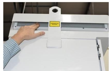
4. Inspect tunnel internally for blockage, through access panels located on front of tunnel above and below VFD. Remove any blockages.
