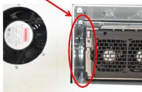
5. Inspect necessary and clean front door air filter (use warm water; dry filter before re-installing). Replace when necessary.
