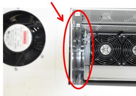
5. Inspect necessary and clean front door air filter (use warm water; dry filter before re-installing).
